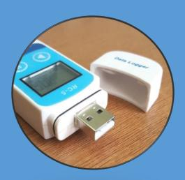
2/ LCD Screen shows temperature and current running status
